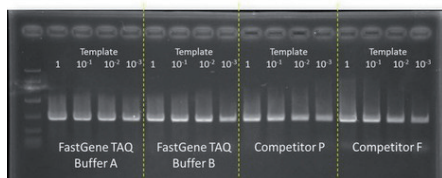
Fig.:1 Reactions (25 µl) were set up according to manufacturer's instructions, amplified fragment is 815 bp. Numbers of cycles were reduced to 25 cycles in order to challenge the PCR enzymes. 10 µl was loaded onto an 1% agarose gel.
